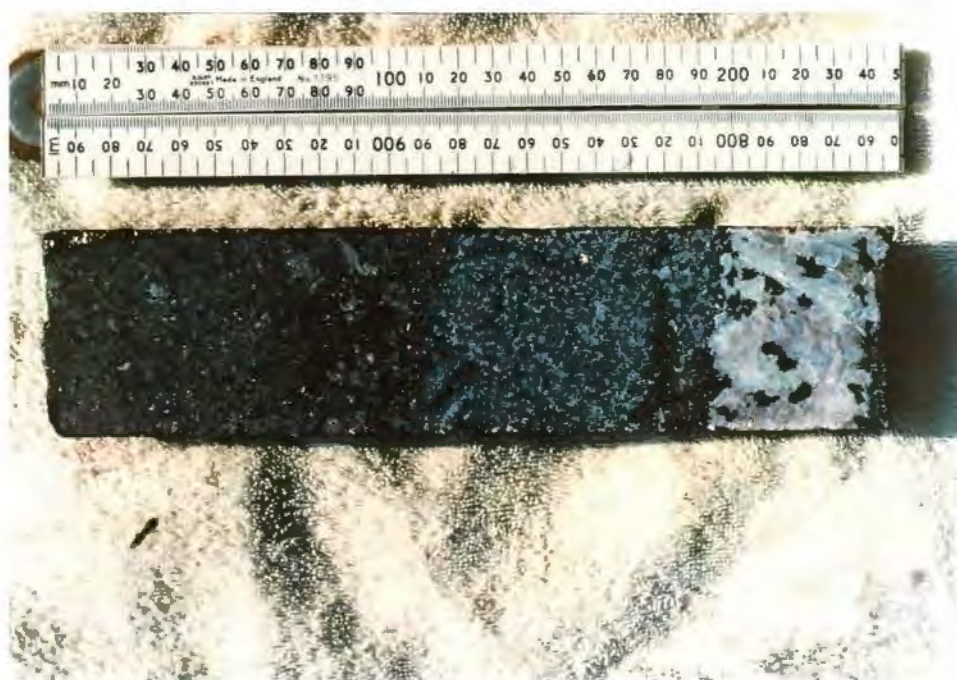
PLATE 12 An intrusive pegmatite vein in magnetite quartzite
