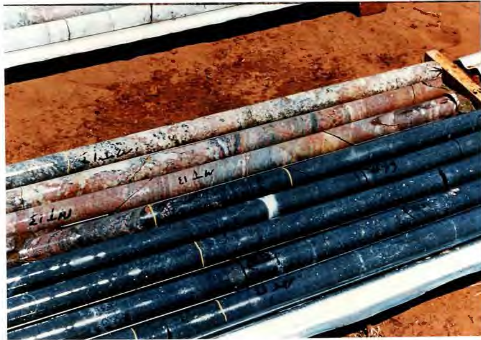
Plate 9 Magnetite quartzite and associated lithologies as seen in drill-core
