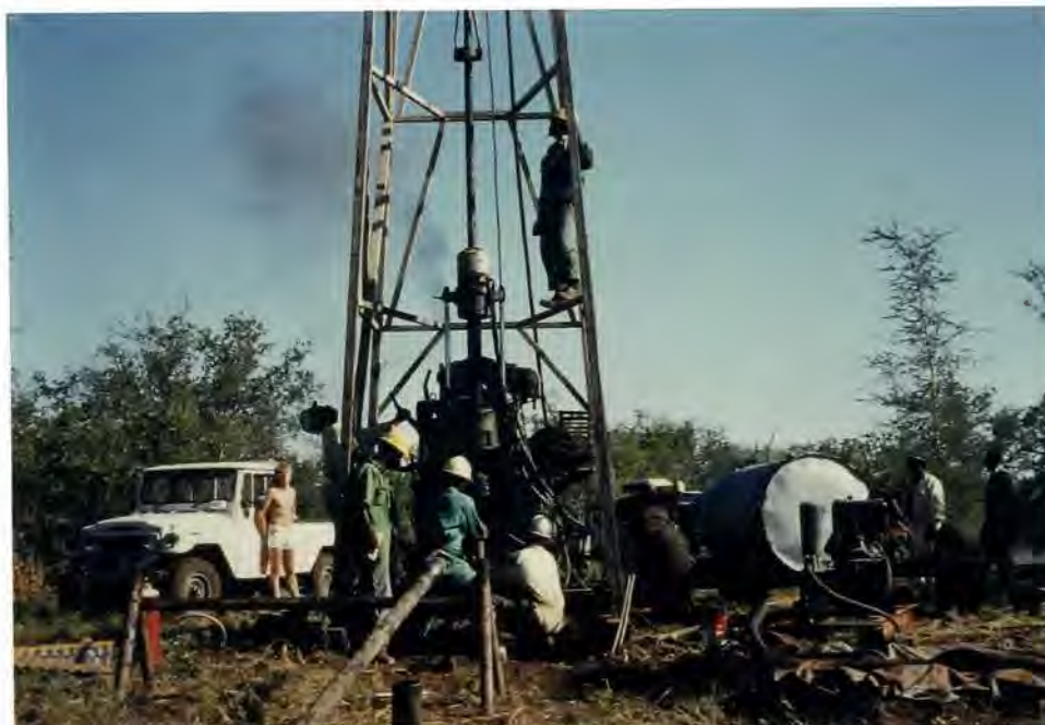
Plate 3 Diamond drilling on grid positions
