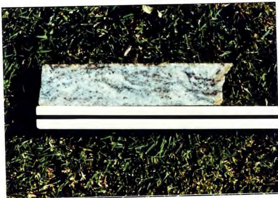
Plate 7 Garnet-quartz-feldspar granulite. The orientation of garnets in planes, may reflect remnant sedimentary layering or metamorphic banding
