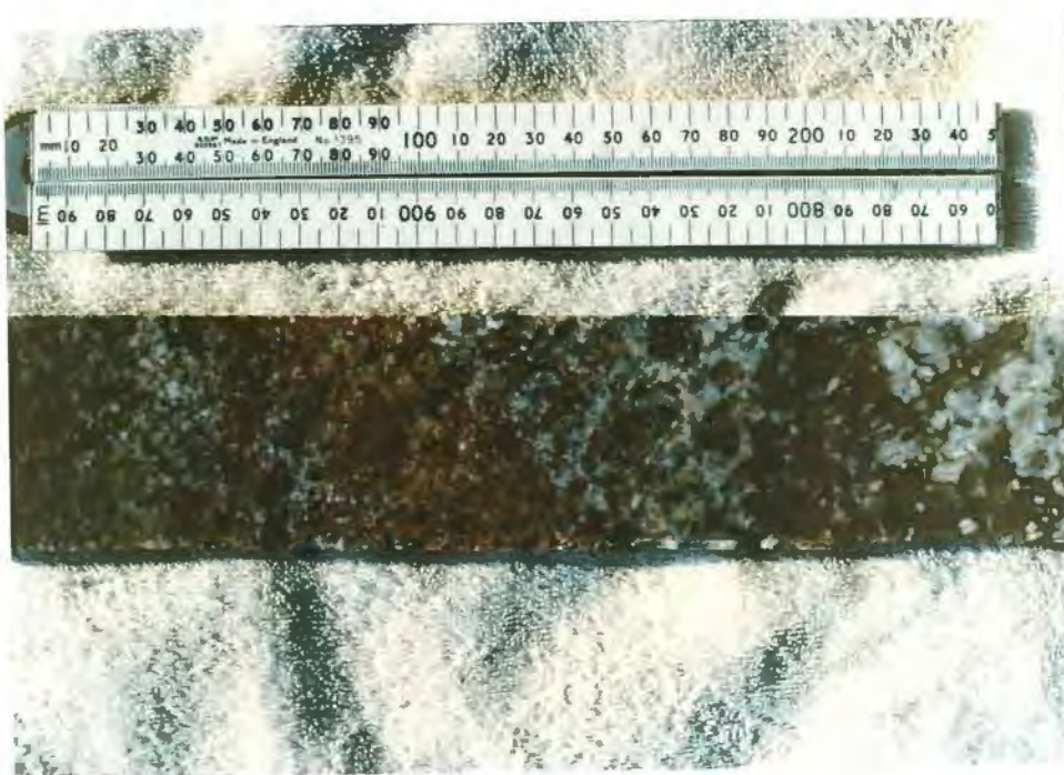
Plate 8 Quartz-feldspar granulite with varying amounts of mafic minerals
