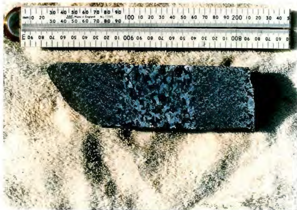
Plate 10 Coarse-grained recrystallization zone in magnetite quartzite (medium-grained)
