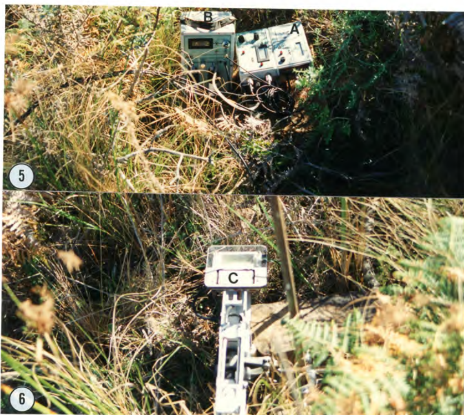
Figs. 5-6. Shows the IRGA set up at a field site (site 2). Fig. 5. Shows the gas analyser (A) and coupled ASUM mass flow meter (B). Fig. 6. Shows the PLC-B- broad leaf chamber (C) containing a leaf.
