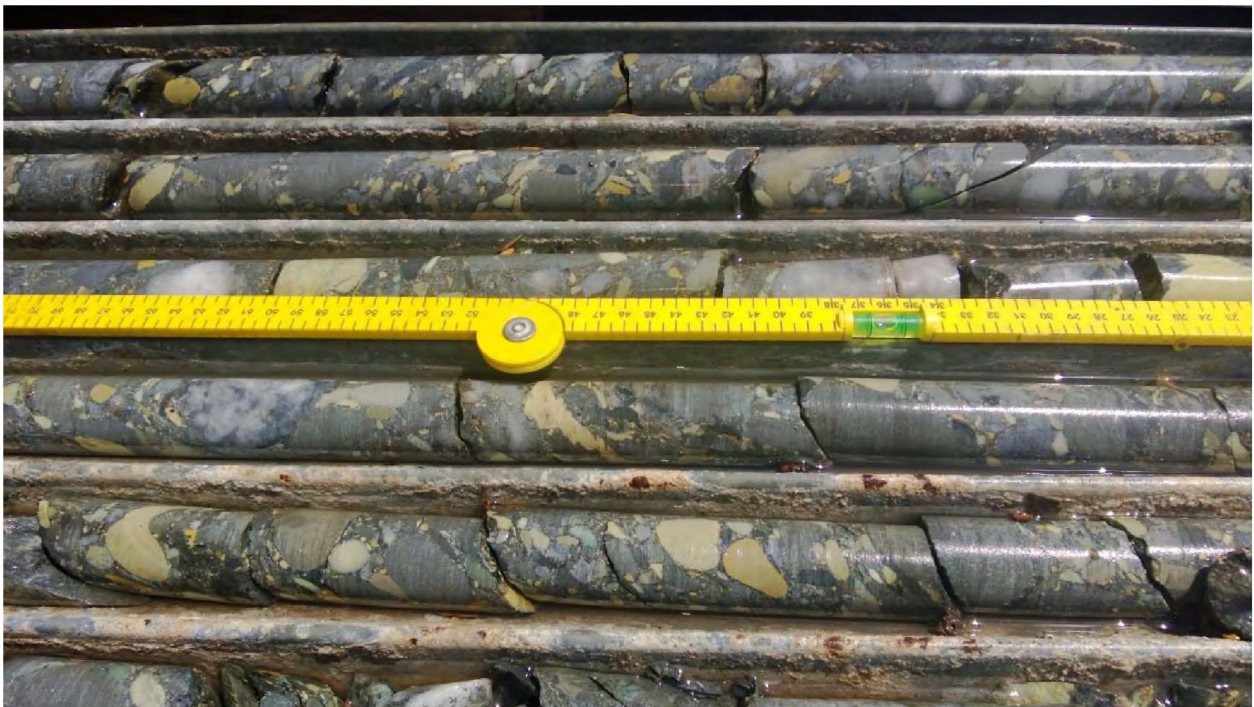
Figure 4.12: Immature VS5 facies with abundant sub-angular to sub-rounded non-durable pebbles (silicified silt and shales, igneous rock fragments, etc). Note the deficiency of large vein quartz pebbles and lack of pyrite mineralization.
