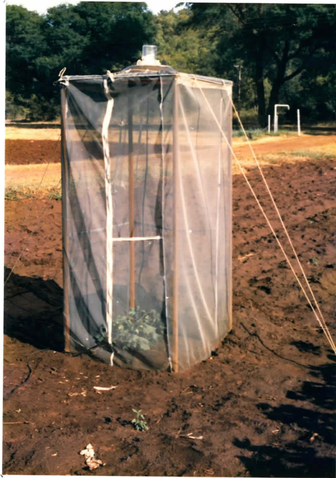
Fig. 2. Black-light trap used to collect live Heliothis armiger moths in the field. The cage (1 x 1 x 1,8 m) was sited at the Hartebeespoort Research Station (Fig. 6), next to a cotton field at the peak flowering stage.
