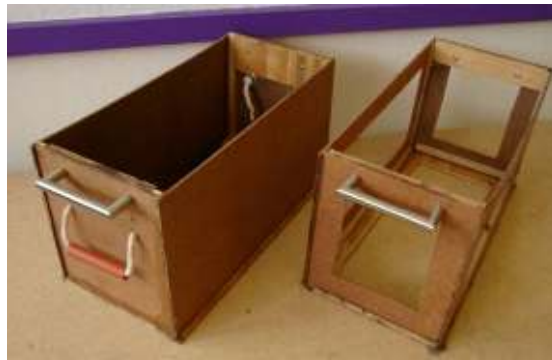
Figure 7: Modified box constituting the lightest loading condition (right) and box used for additional two loading conditions (left).
