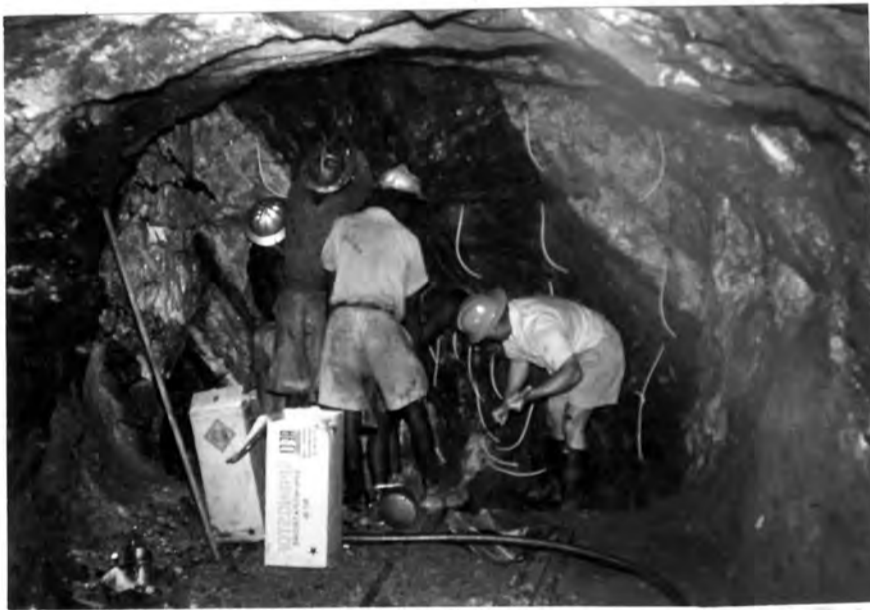
Face of the advancing Main Adit Drive showing the dip of the ore-body at 60^{\circ} to the south. A band of dark graphitic and partly schistose granulite is seen between coarse white calcite on the hangingwall side and pink calcareous granulite. The coarse sulphide mineralisation can be seen glinting in the light.
