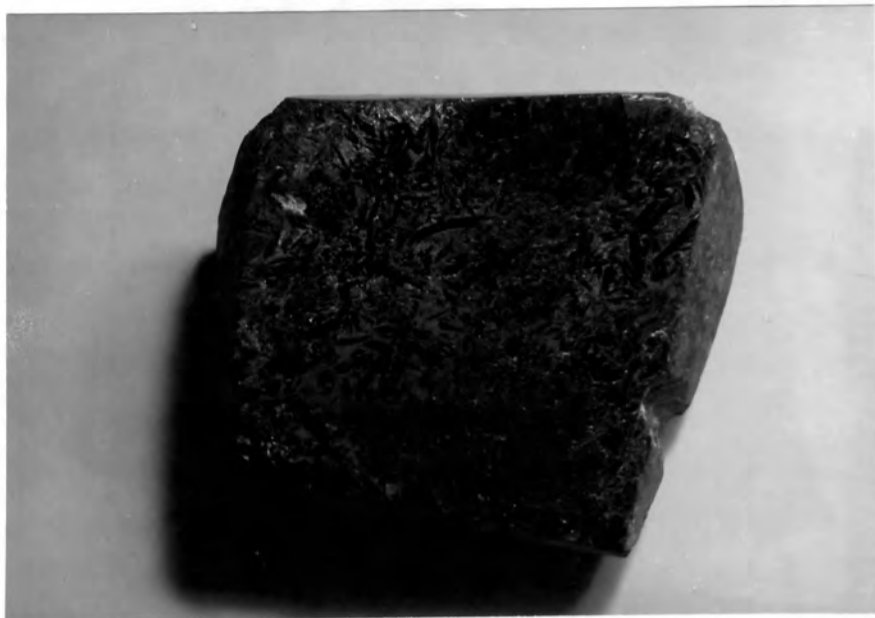
Massive sulphide ore (pyrrhotite, chalcopyrite, cubanite) with green bladed hydrothermal hornblende from Main Adit Drive.
