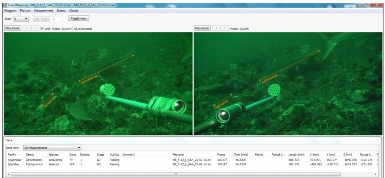
Appendix 2.2: Measuring the length of fish, and their range from the cameras, using the video analysis software EventMeasure ( www.seagis.com.au ).
