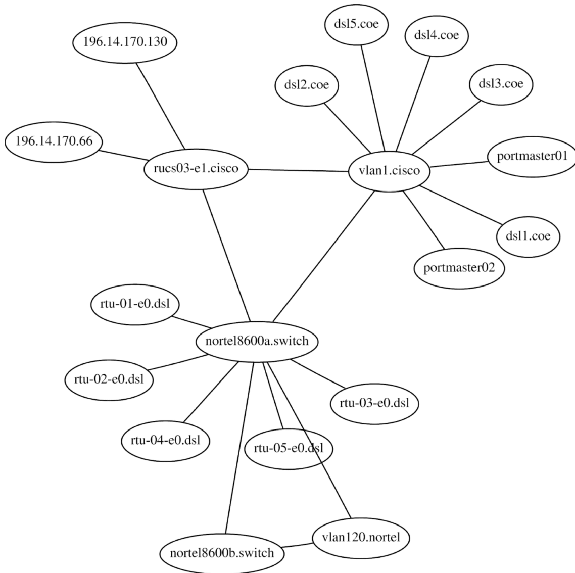
Figure 4-1. Topological map of Rhodes University’s network
