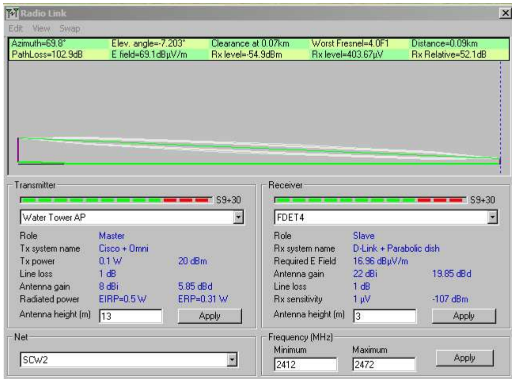
Figure C.6: The Fresnel zone at FDET4
