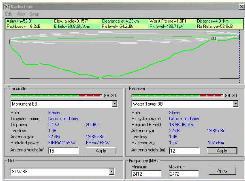
Figure 6.18: Fresnel zone diffraction on the link between the Monument backbone AP and the bridge at the water tower.
