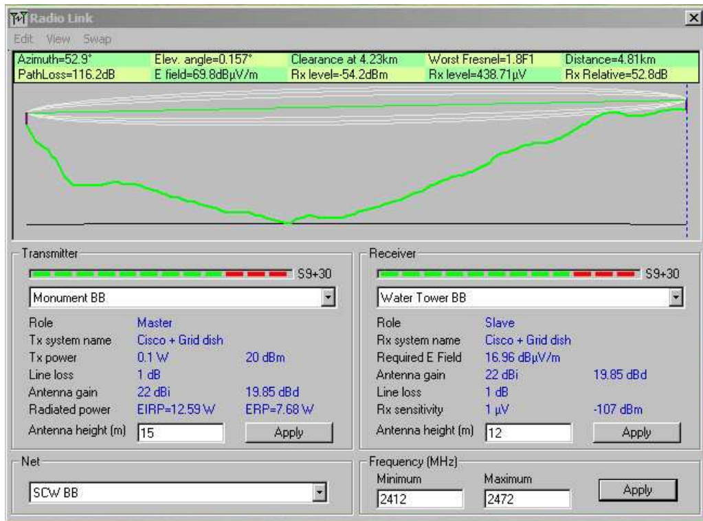
Figure 7.2: The Fresnel zones from the Monument backbone AP to the water tower bridge backbone, using 2.4 GHz spectrum.
