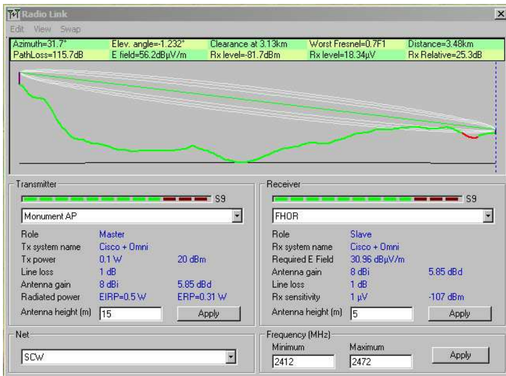
Figure C.4: The Fresnel zone at FHOR
