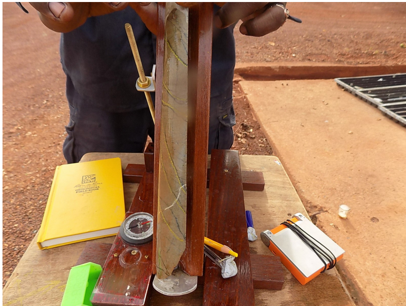
Figure 5. Photo of NW trending Veins on half cores.
