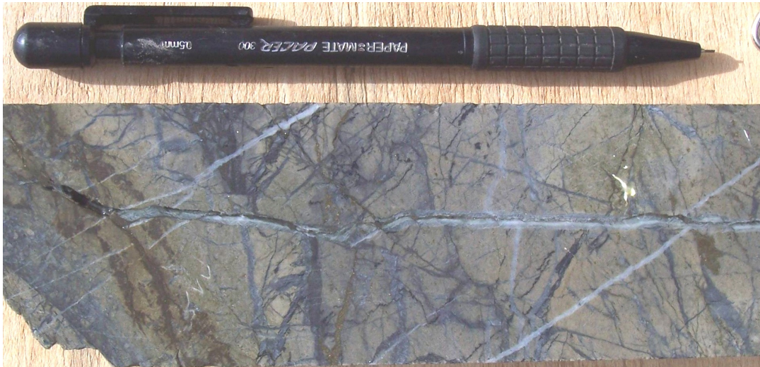
Figure 21. Stockwork ore in Basalt (after Standing, 2007).
