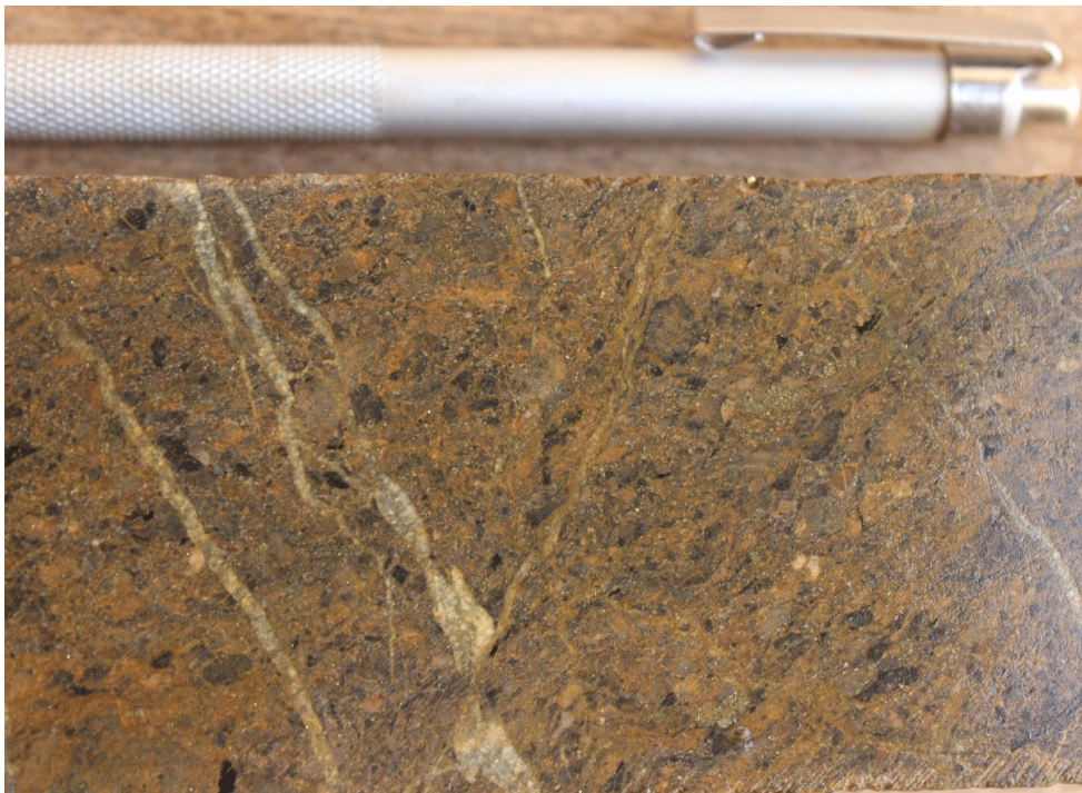
Figure 24. Disseminated pyrite in altered greywacke. Photo taken from Syama core library.
