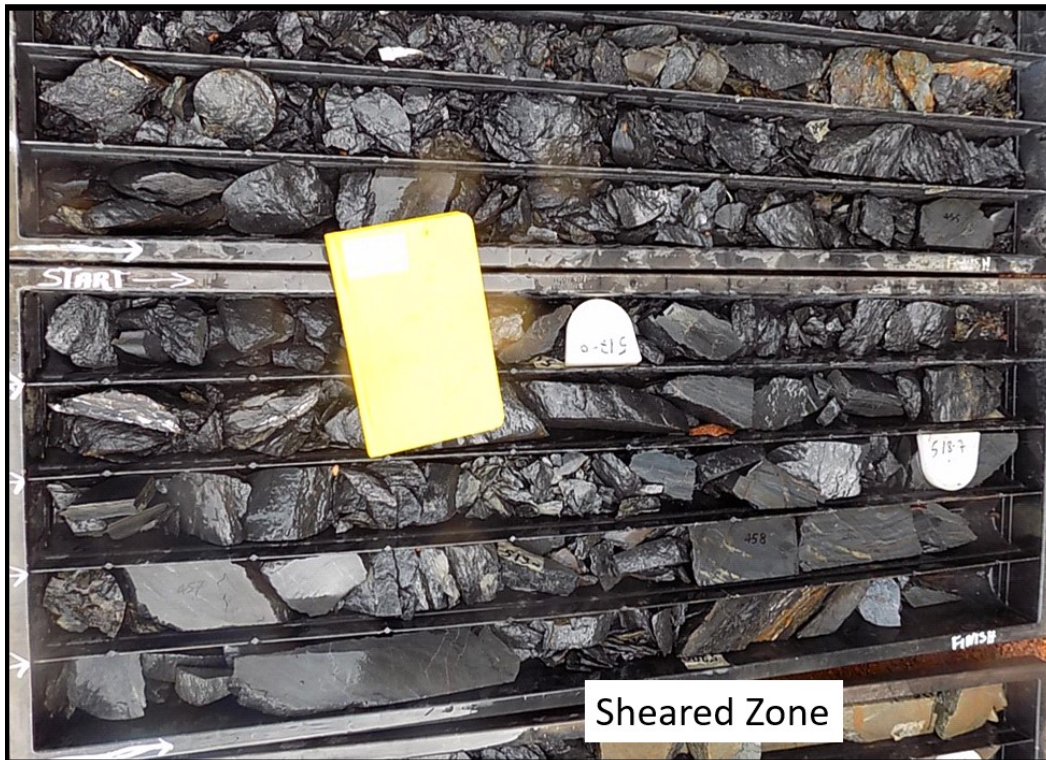
Figure 19. Sheared Carbonaceous Shale (Hole ID: SYDD432). Photo taken on half core.
