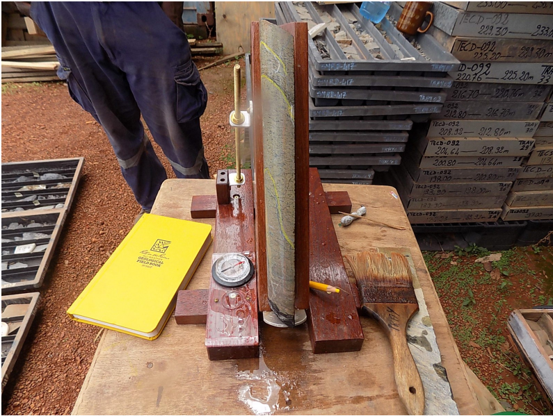
Figure 3. Photo of NW trending Foliation on half cores.
