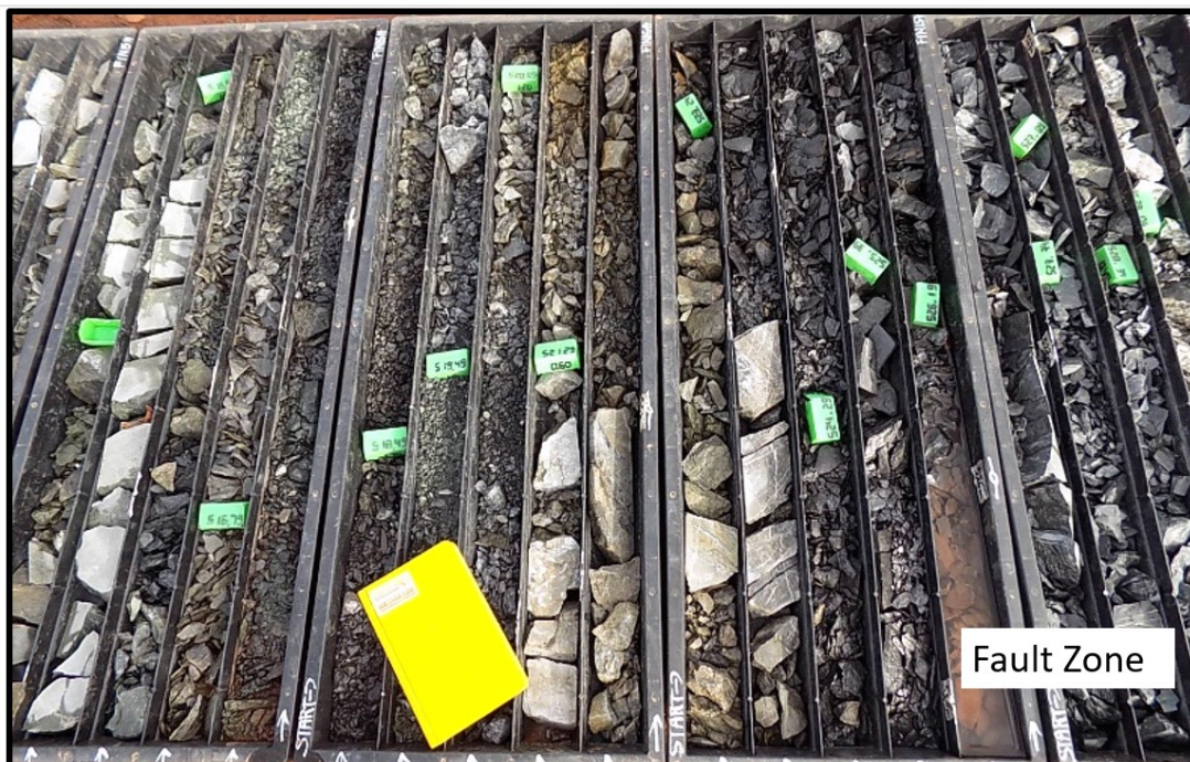
Figure 20. Brittle fault zone affecting more competent basalt, lamprophyre and silicified carbonaceous shale, (Hole ID: SYDD432). Photo taken on half core.
