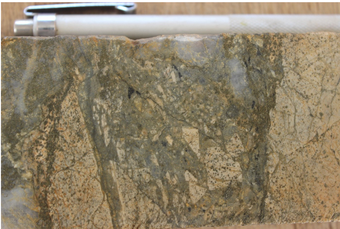
Figure 22. Breccia ore zone. Photo taken from Syama core library.
