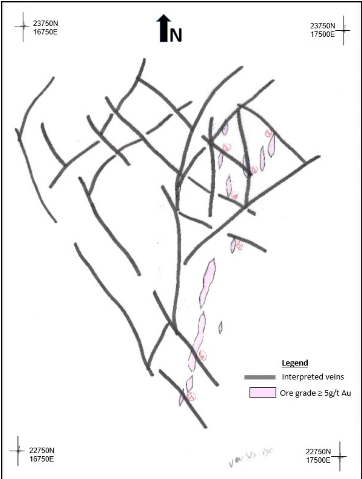
Figure 54. High-grade ore equal or above 5g/t Au versus Veins at mine level 1100mRL.
