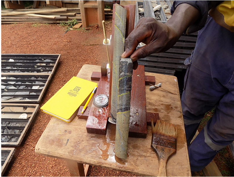
Figure 4. Photo of NW trending Shears on half cores.
