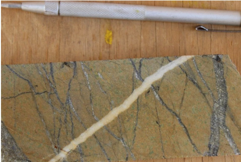
Figure 23. Sheeted veinlet ore. Photo taken from Syama core library.
