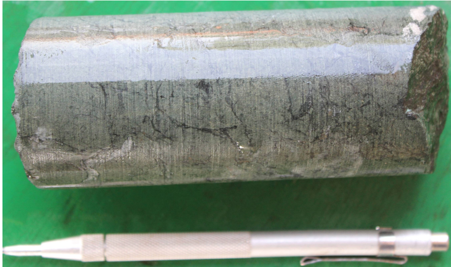
Figure 13. Basalt unit with chlorite-calcite alteration. Photo taken from Syama core library.
