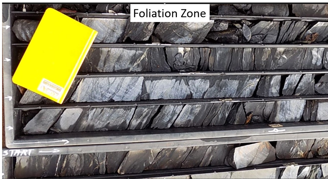
Figure 18. Foliated Carbonaceous Siltstone (Hole ID: SYDD432). Photo taken on half core.
