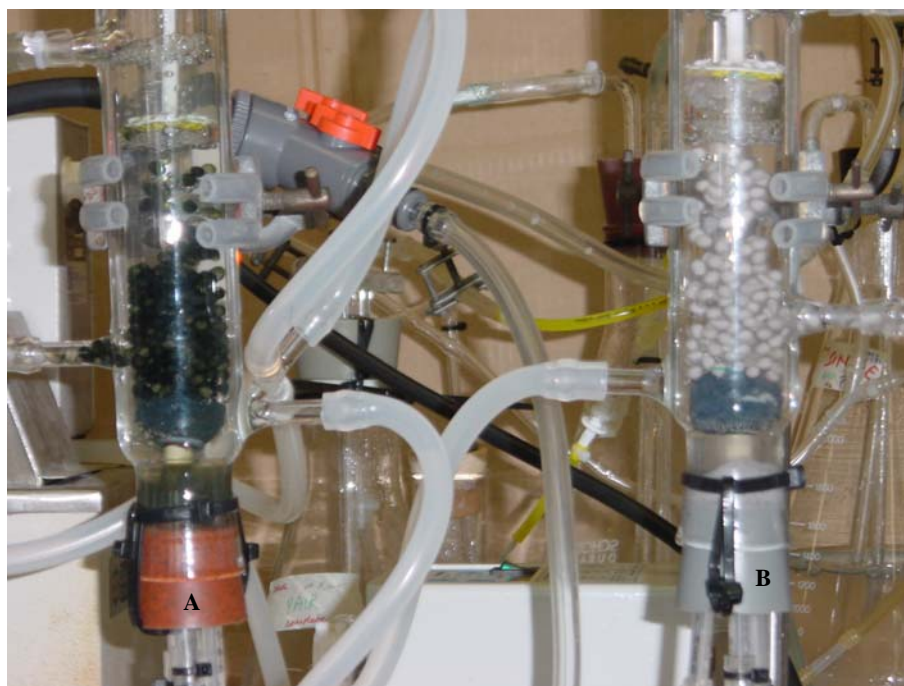
Figure 5.3: Continuous up-flow packed columns with calcium-alginate-xanthan gum encapsulated SRB. A = column with an inorganic influent stream spiked with copper where the SRB capsules have gone black in colour; B = column where the influent does not contain copper, and the SRB capsules are grey in colour.
