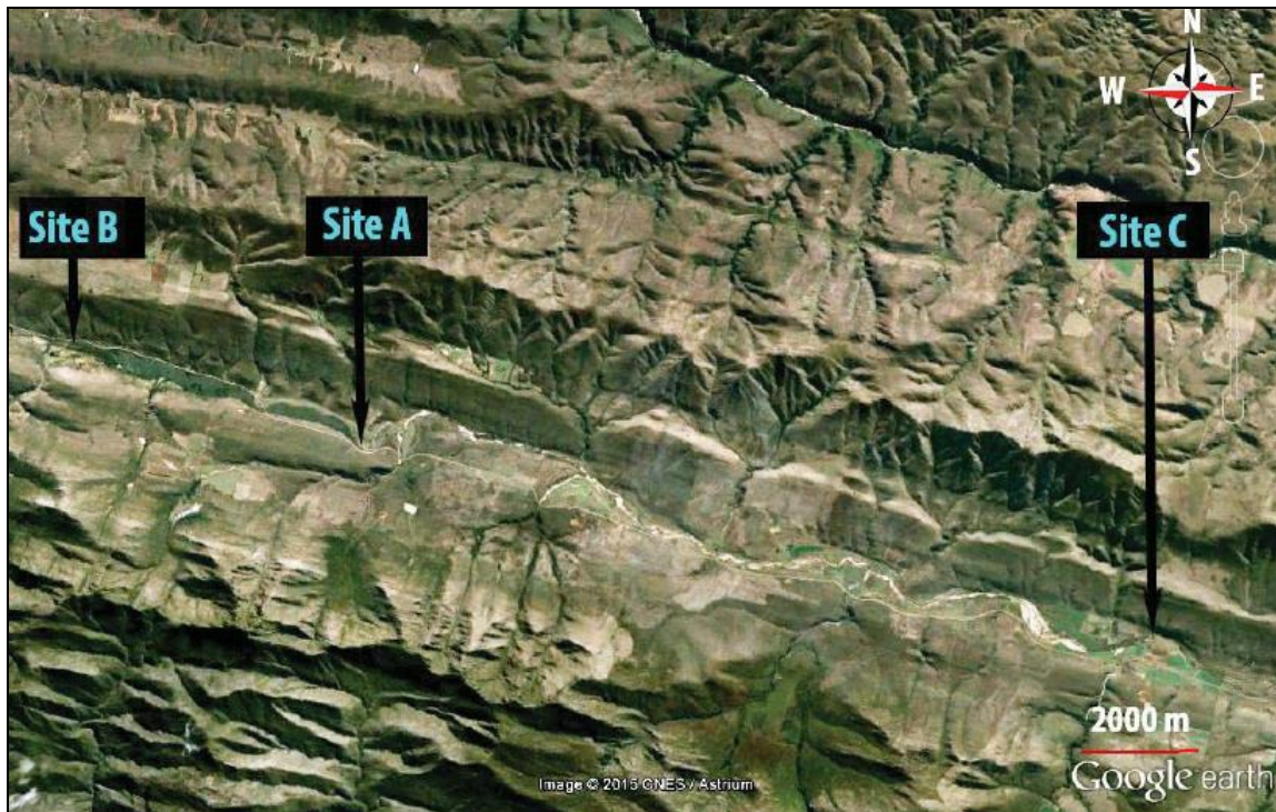
Figure 3.12 Sites of sub-surface water level measurement using piezometers installed adjacent to erosion control structures (at site A) and potential future structures (site B and C) (De Haan, 2016).
