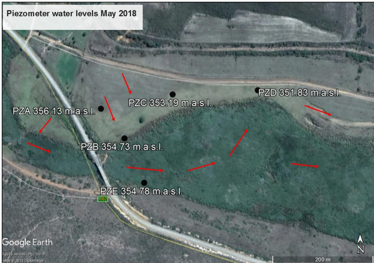
Figure 5.17 Proposed sub-surface flow directions at the Kompanjiesdrif wetland with water levels measured in May 2018.
