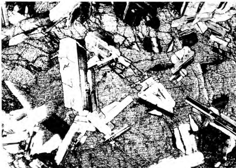
Fig. 2: Photomicrograph showing poikilophitic texture in dolerite. X 12, crossed nicols. Laths of plagioclase (pl) are wholly enclosed by large crystal of pyroxene (py).
