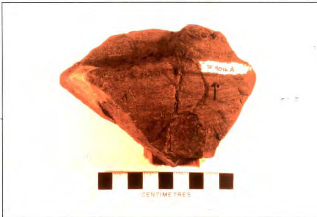
Figure 18. Handspecimen showing a vertical clay-filled root trace within a laminated sandstone (Middle mudrock sequence, Cr horizon, 31.84 m from the top of the sequence, Appendices 2 and 3).
