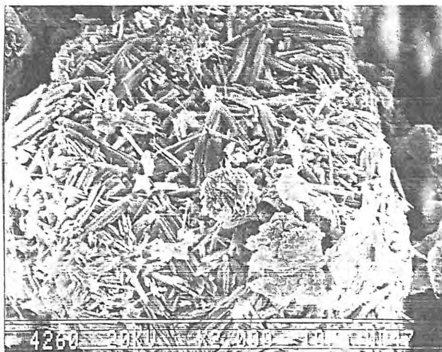
Fig. 7.37a. Scanning electron micrograph of a \text{WO}_3 /graphite mixture after 60 min at 935^\circ\text{C} .
