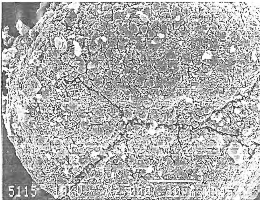
Fig. 9.5a. Scanning electron micrograph of a \text{WO}_3 /graphite mixture (1:4 mole ratio) after heating for 2 min at 875^\circ\text{C} in hydrogen flowing at 200\text{ mL min}^{-1} .
