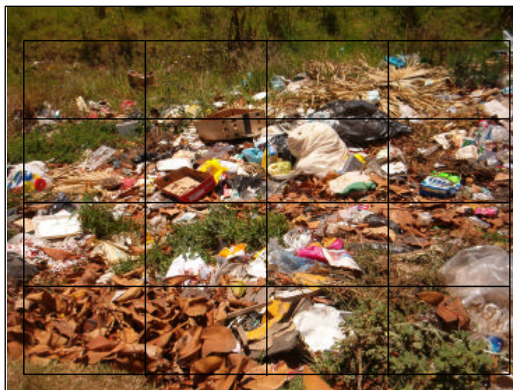
Figure 3.2: A grid of 16 squares was used to estimate the percentage cover of solid waste in each quadrat.
