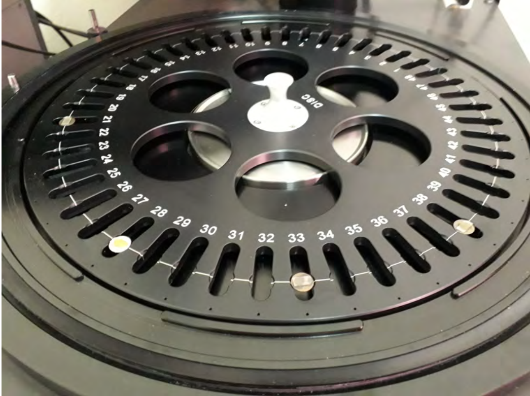
Figure 5.4: A picture of the carousel with samples of \alpha\text{-Al}_2\text{O}_3\text{:C,Mg} at positions 21, 28, 33 and 38 respectively. The unannealed sample is at position 28 whereas the samples at positions 33, 38 and 21 are annealed at 700, 900 and 1200°C for 15 minutes respectively.
