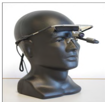
Figure 8: The head unit of the Dikablis eye-tracking system
