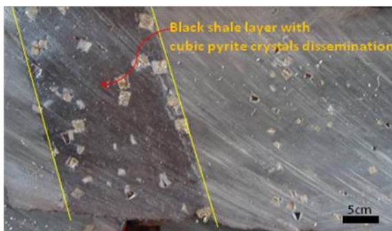
Figure 3.3.2: very fine-grained black shale interbedded with medium to fine-grained siltstone with cubic pyrite crystals; note these types of pyrite crystals are not associated to gold mineralization.
