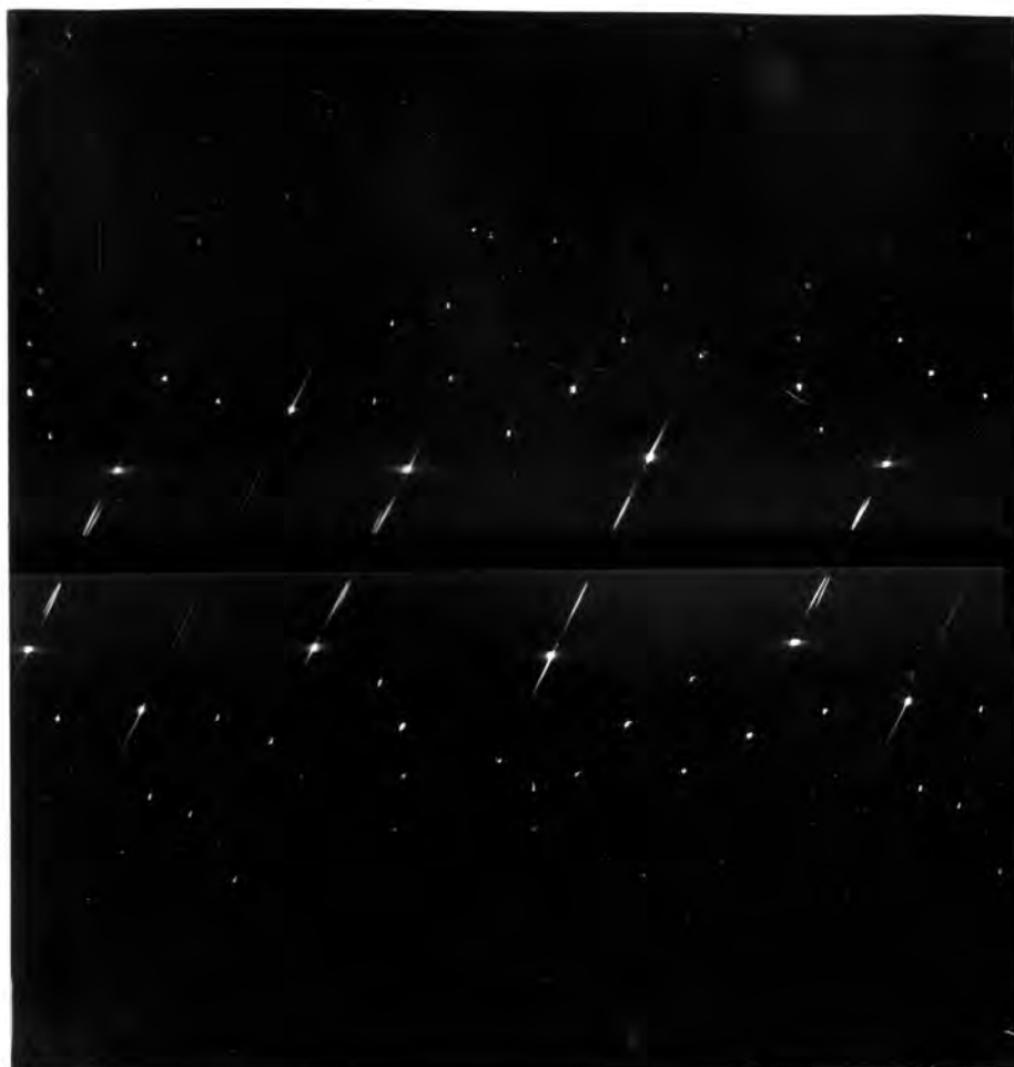
PLATE 7. Zero-layer Weissberg photograph. Crystal mounted along c , (filtered copper radiation).
