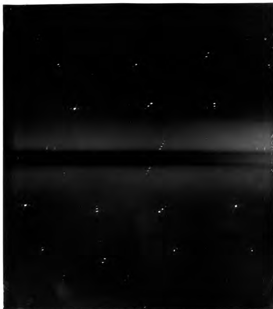
PLATE 3. Zero-layer Weissenberg photograph. Crystal mounted along b , (filtered cobalt radiation).
