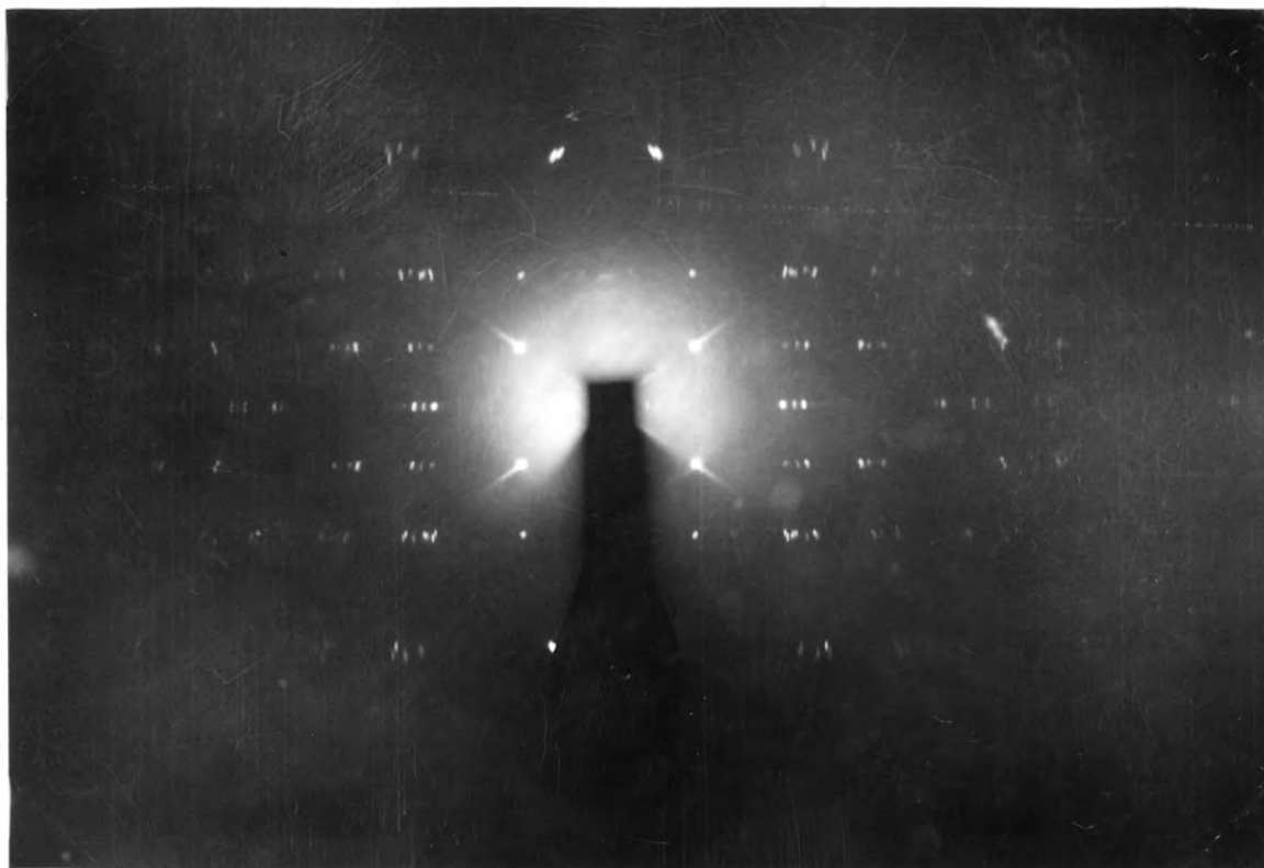
PLATE 2. Rotation photograph about b , (filtered cobalt radiation).
