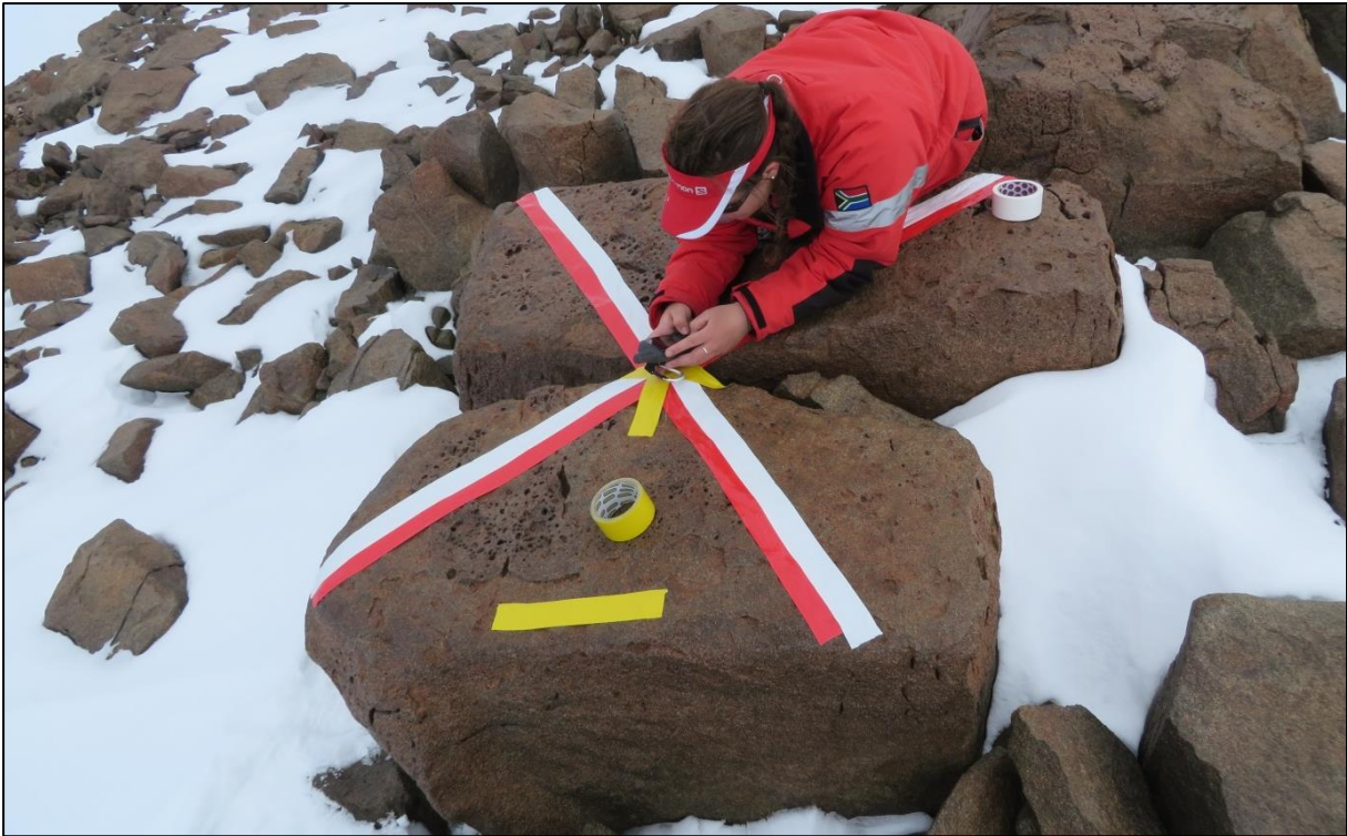
Figure 13: Crosses used as ground control points
