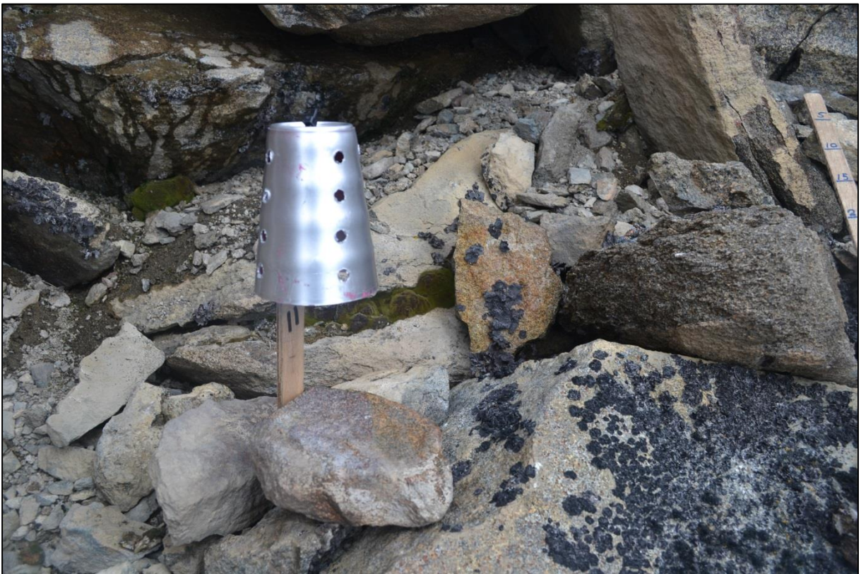
Figure 11: Radiation shield set up for the iButtons
