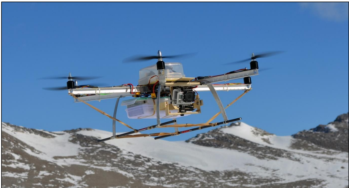
Figure 12: The hexacopter used for capturing aerial imagery
