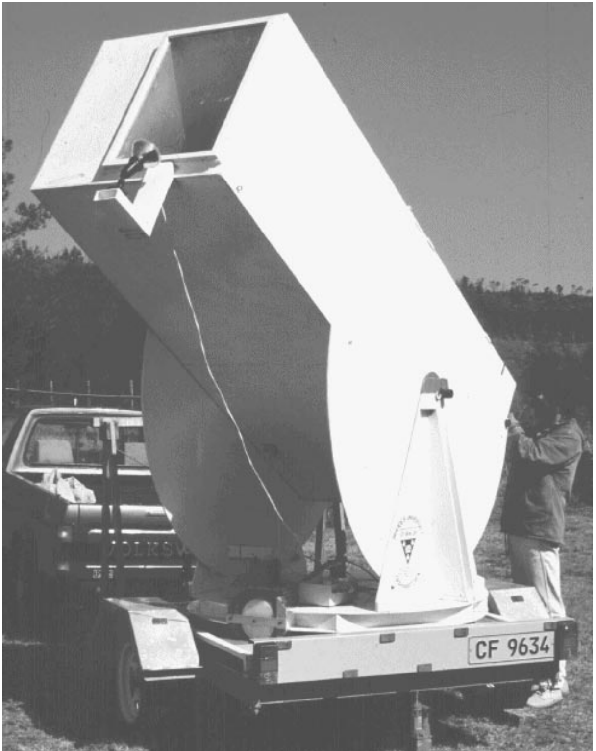
Figure 9.3: The portable 2.3 GHz horn telescope mounted on its road trailer. The scale of the instrument can be ascertained from the height of the author (who is 1.73-m tall). The spotlight directed towards the mouth of the horn antenna is intended to keep the mylar radome clear of condensation. The motorized azimuth drive wheel is visible on the near-side of the azimuth turntable. The entire receiver system is enclosed within the rectangular box, which is lined with thermal insulation.
