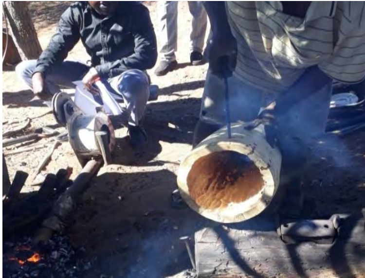
Figure 6.7: Using bradawl- Munho to drill a hole for pegging
