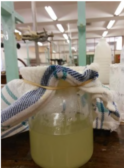
Figure 6.1.2.1 Photograph of cloth and beaker showing a kitchen chemistry method of gravity filtration
