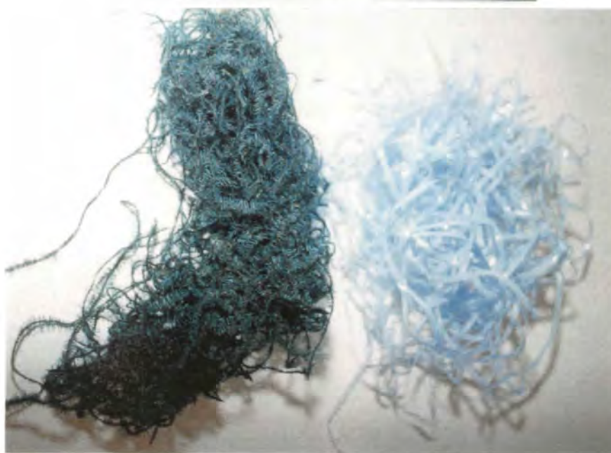
2.4.1 Photographs of artificial media:(a) Wool mop on 5mm plastic mesh false bottom; (b) Strip plastic and shredded shade cloth.
