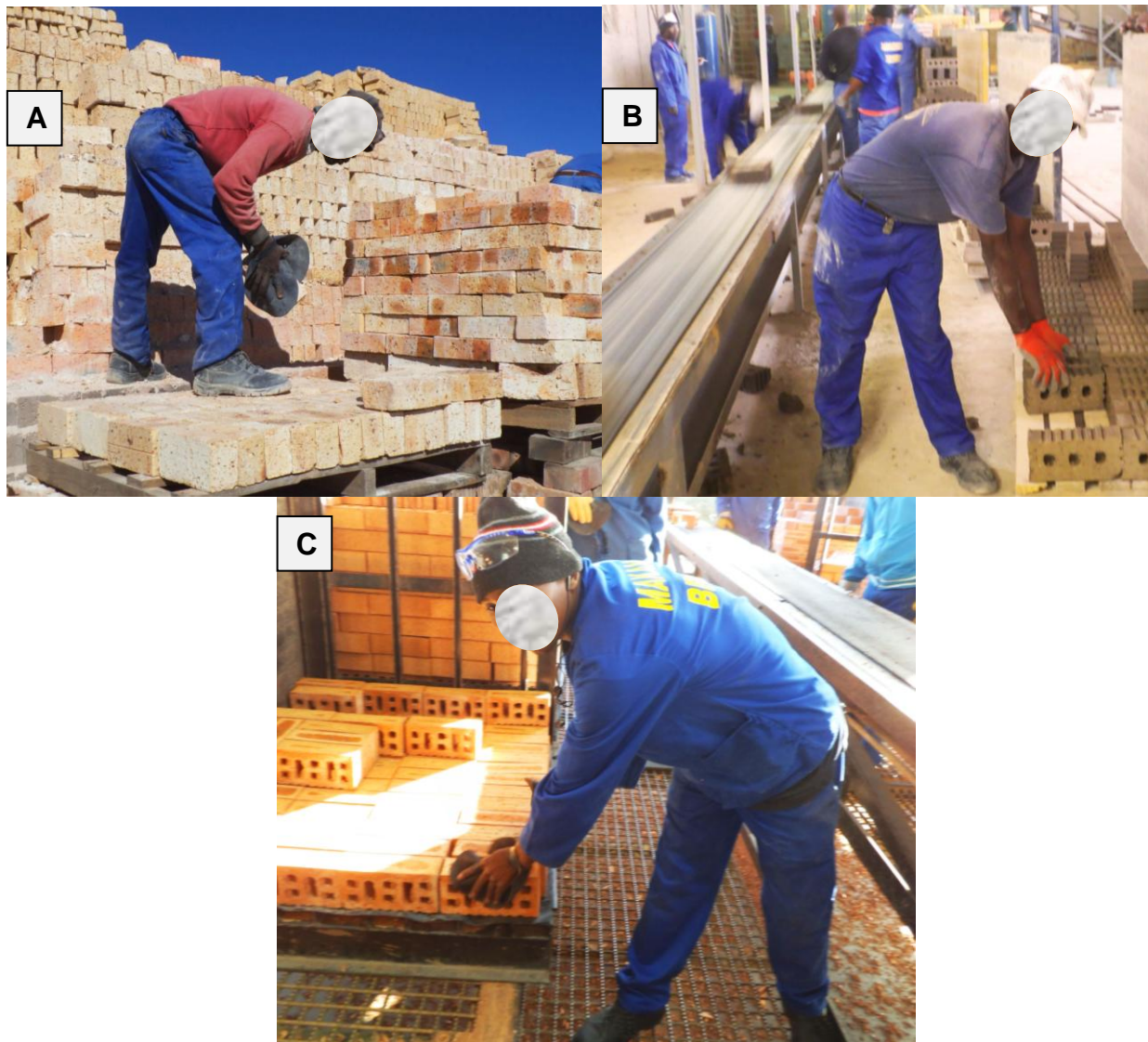
Figure 8: Images of the three MMH palletising tasks; A) Clay Dry Brick (CDB), B) Clay Wet Brick (CWB) and C) Kiln Dry Brick (KDB).
