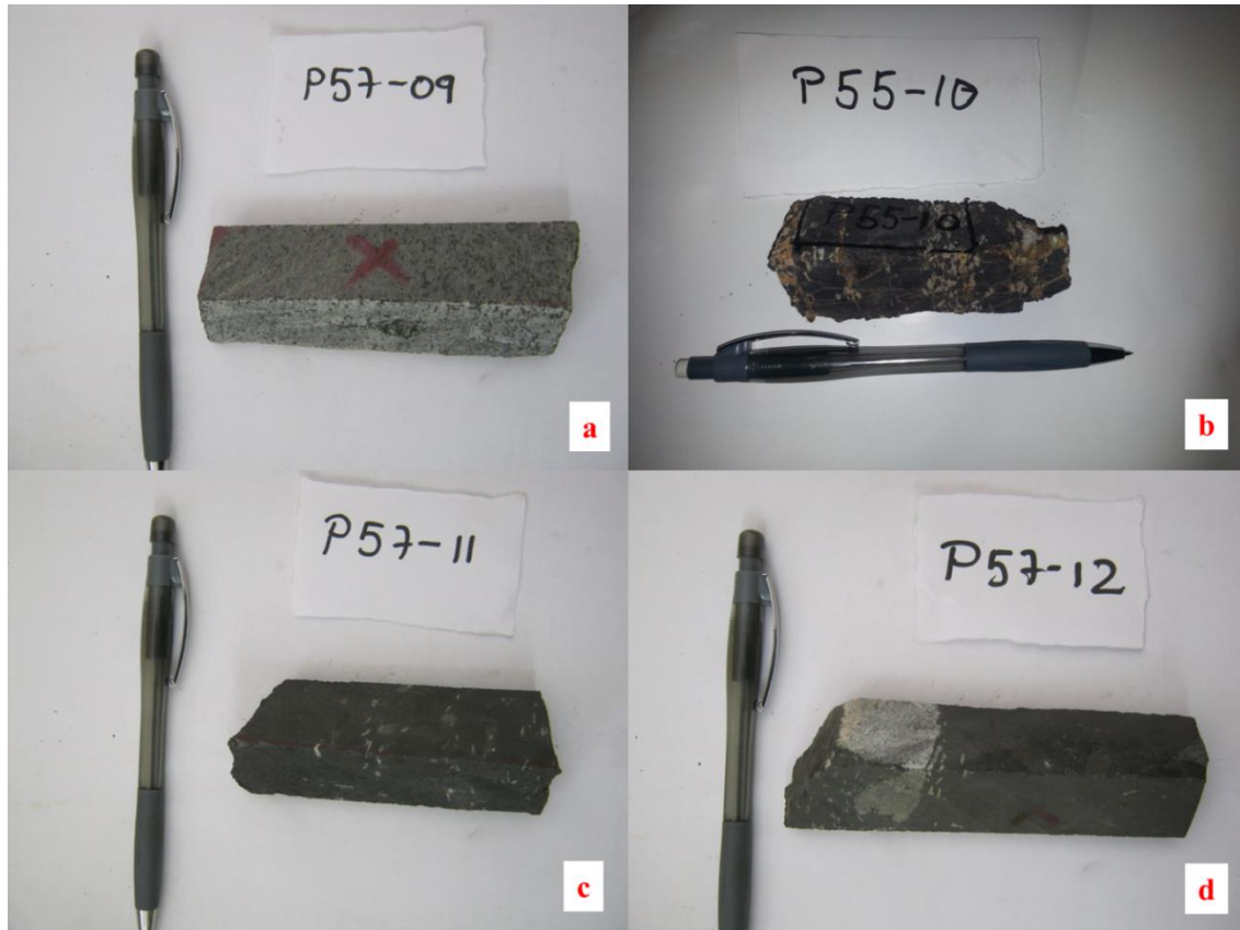
Figure 5 Quarter core samples which were prepared into polished thin sections. (a) Magnetite anorthosite parting between MAG 04 and MAG 03 in P57 (b) magnetite-plagioclase cumulate (c) massive magnetite with minor plagioclase (d) massive magnetite with plagioclase laths
