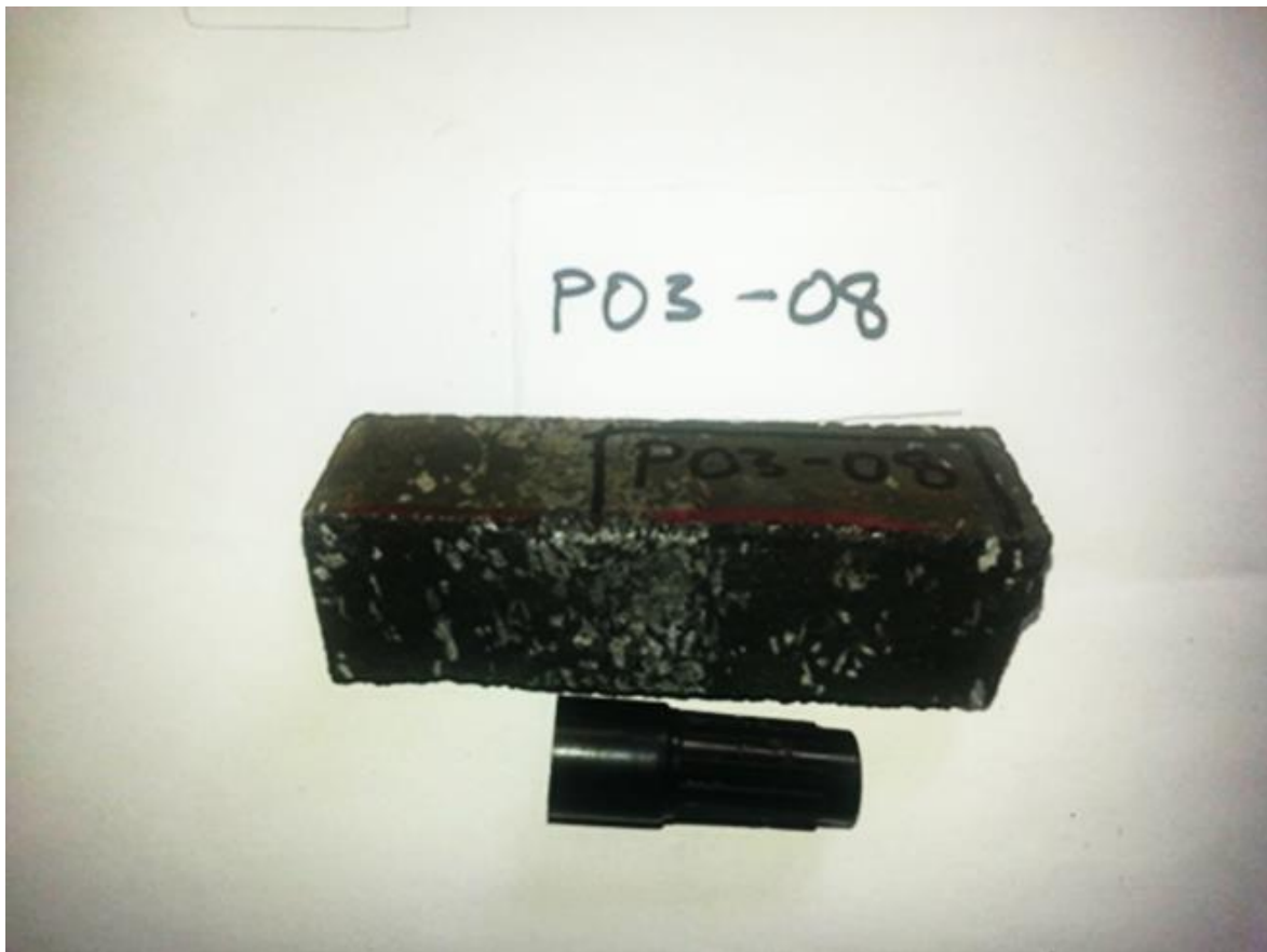
Figure 17 Orthocumulate titanomagnetite-silicate ore from the Upper Zone. The light silicates are largely plagioclase. Note the preferential orientation of plagioclase.
