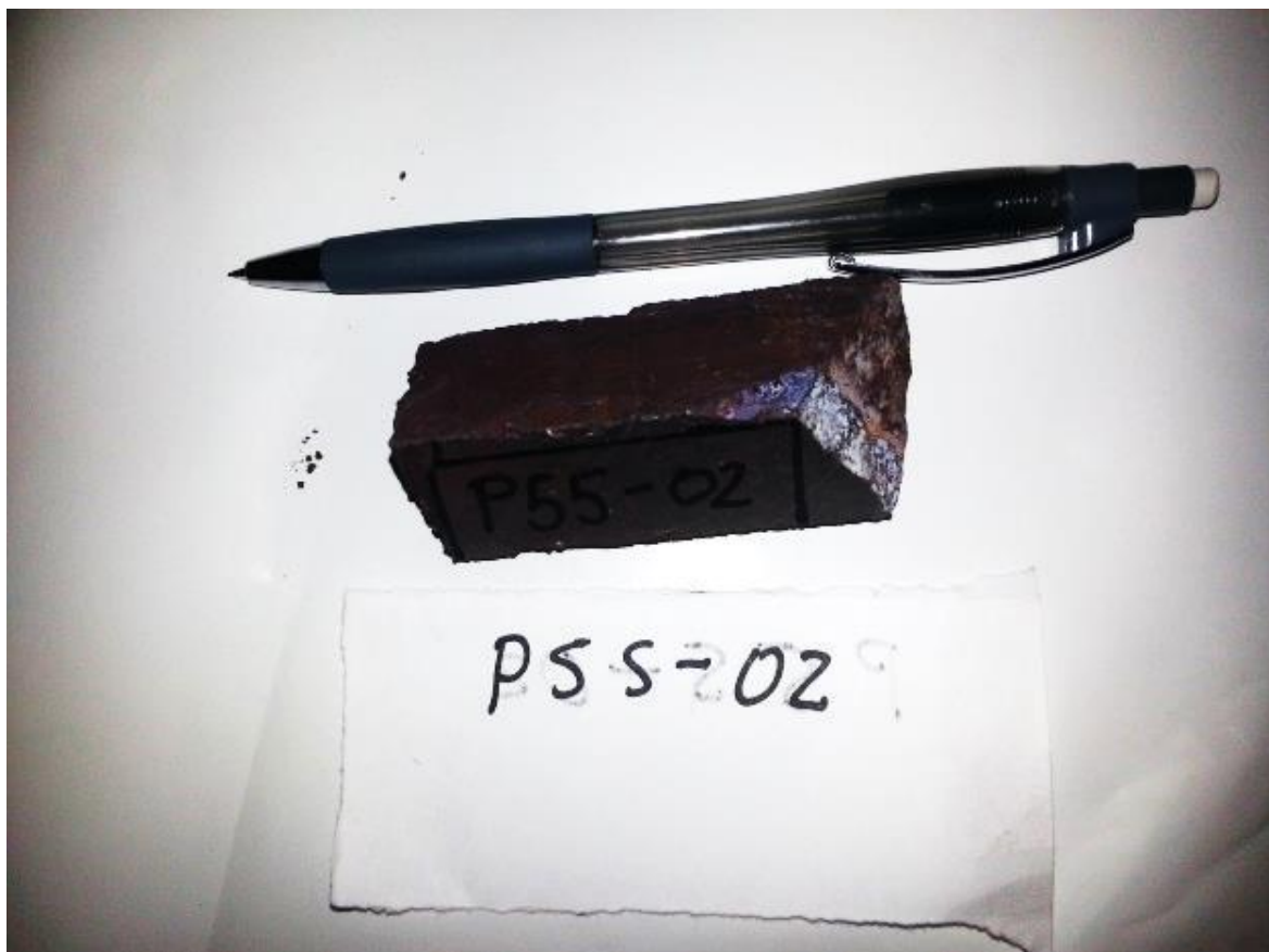
Figure 16 Massive (adcumulate) titanomagnetite ore from the Upper zone magnetite.
