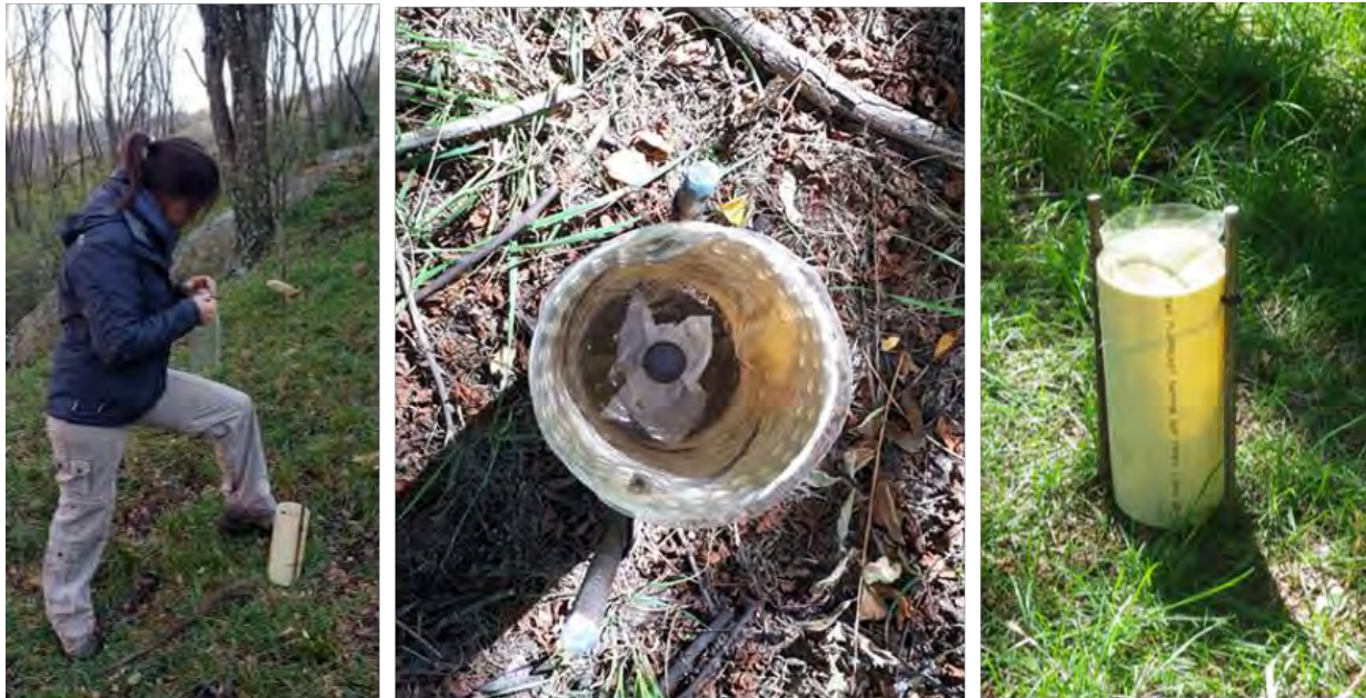
Figure 2.3. The seed rain traps mounted below trees to collect seeds falling from Robinia pseudoacacia .
