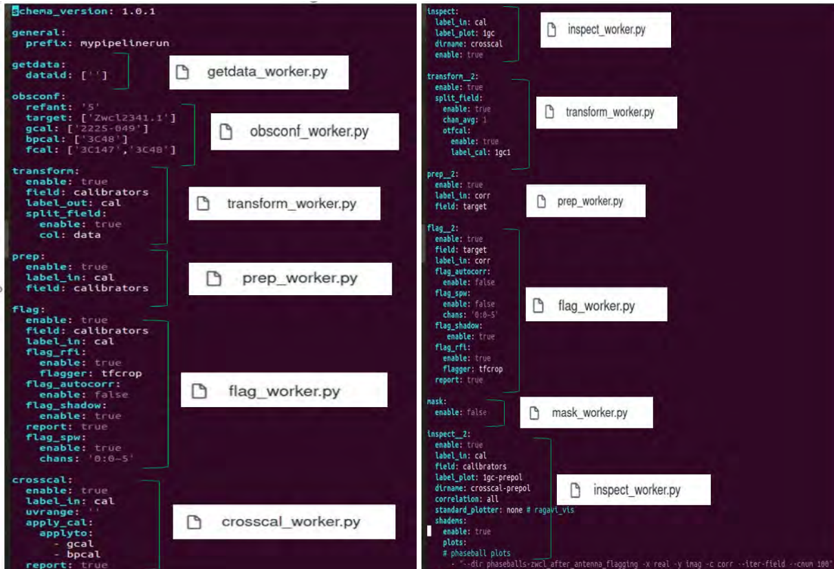
Figure G.1: CARACal example .yml file showing the workers on the left, each encapsulated by a green right bracket. The corresponding worker .py script is shown in the white box on the right of each worker. The tasks are indented to the right under each worker name. The parameters for each worker are shown in purple.
