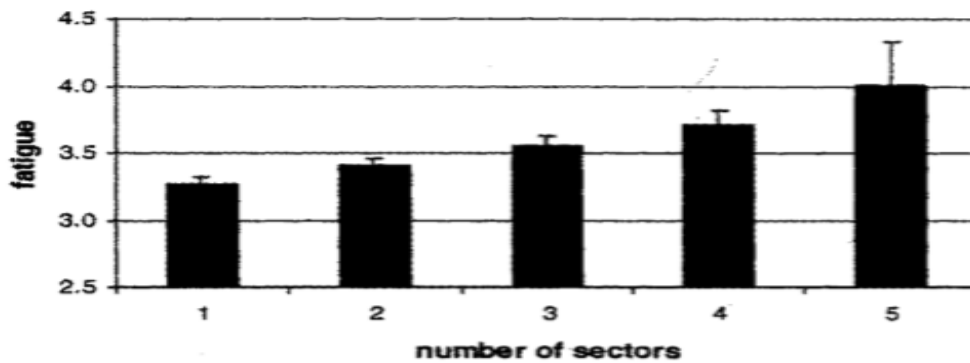
Figure 10: The effect of the number of consecutive flight sectors on fatigue levels. Fatigue ratings were based on the Samn-Perelli 7-point fatigue scale 1 = “Fully alert, wide awake”; 2 = “Very; lively, responsive, but not at peak”; 3 = “Okay, somewhat fresh”; 4 = “A little tired, less than fresh”; 5 = “Moderately tired, let down”; 6 = “Extremely tired, very difficult to concentrate”; 7 = “Completely exhausted, unable to function effectively” ( taken from Spencer and Robertson, 2002, p. 11)
