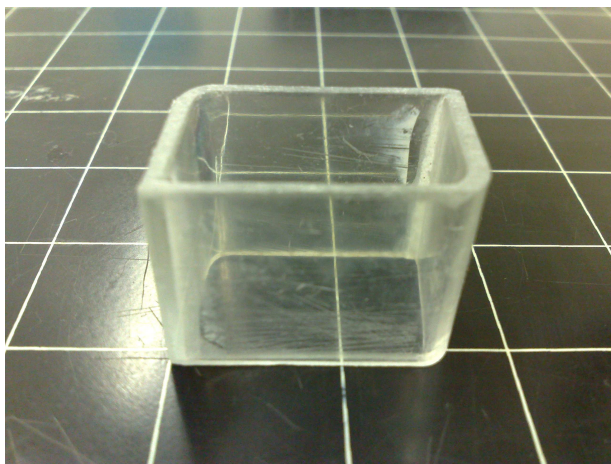
Figure 7.7. PVC custom-made chamber
