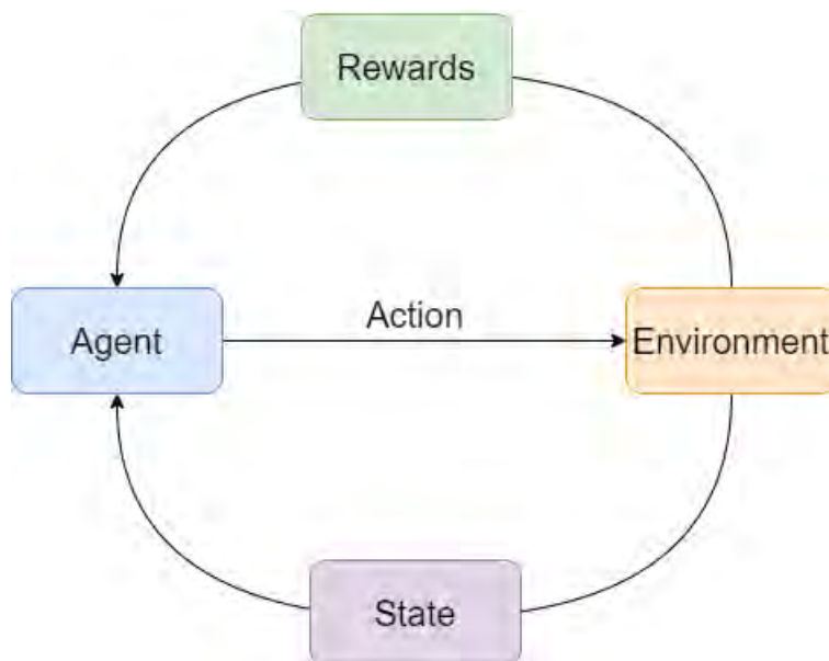
Figure 2.21: The reinforcement learning loop, where an agent interacts with the environment by taking actions. The environment responds by updating the state and providing rewards, guiding the agent’s actions to maximize performance.
