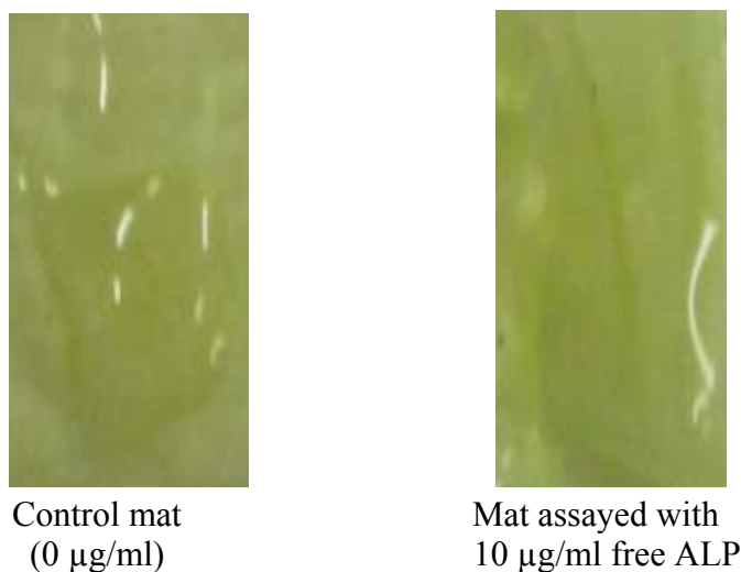
Figure 5.17a: ALP assaying on nylon-pNPP nanofiber mats after 80 °C heat treatment. The mat turned yellow after treatment meaning the 10 µg/ml ALP standard was not responsible for the yellow colour observed.
