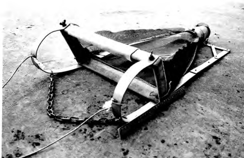
Figure 5. Net used for sampling in study site. Dimensions are: net opening 370 x 180 mm; mesh size 1,3 mm; net length 570 mm; diameter of cod end 80 mm.
