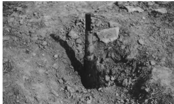
Figure 110: Heave meter (Wang & French 1995: 339).
