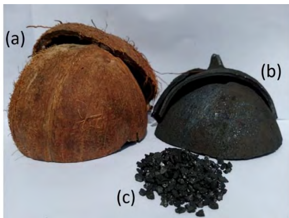
Fig. 3.7: Transformation stages of coconut shell starting from (a) the raw coconut shells to (b) carbonized shells and (c) the granulated form
