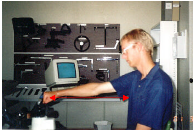
Figure 14: Subject seated knuckle distance from the control being tested, with the axis of the control aligned, in the transverse plane, with the subject's xiphoid process when seated (see red arrow).
