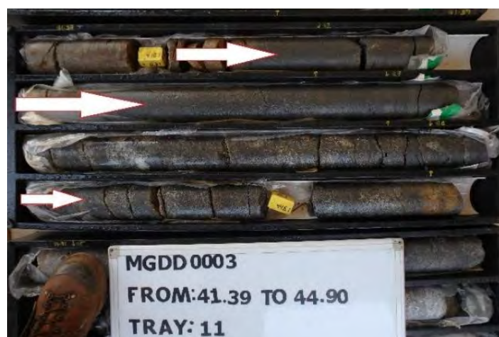
Figure 18: Malingunde diamond drilling (MGDD0003) core tray
