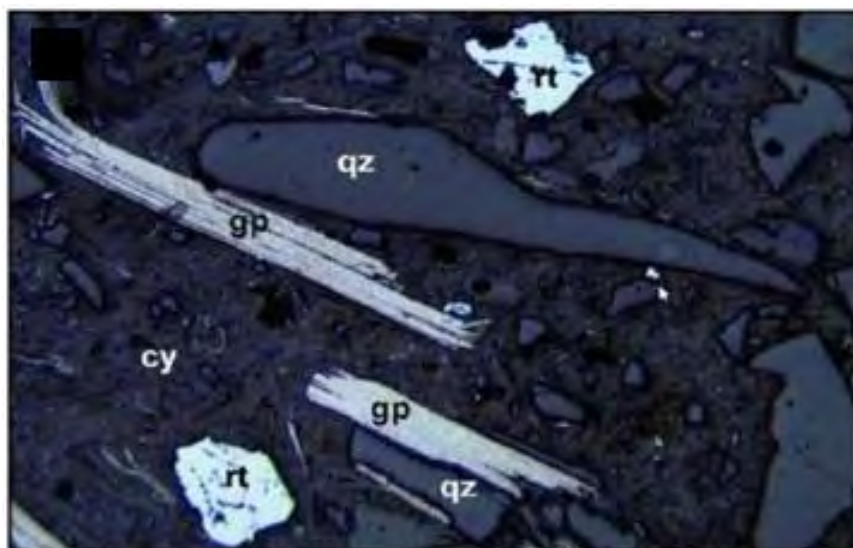
Figure 21: Thin section of one of the saprolite samples for the Malingunde project (Edited from SML, 2018)
