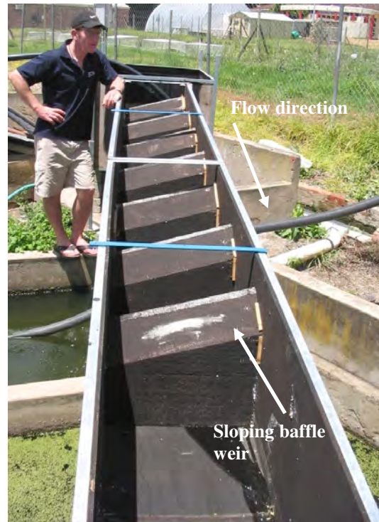
Plate 2.2: Sloping Baffle Fishway used during experiments.
