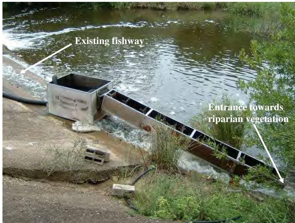
Plate 2.4: Vertical Slot Fishway position 2, placed over existing fishway.
