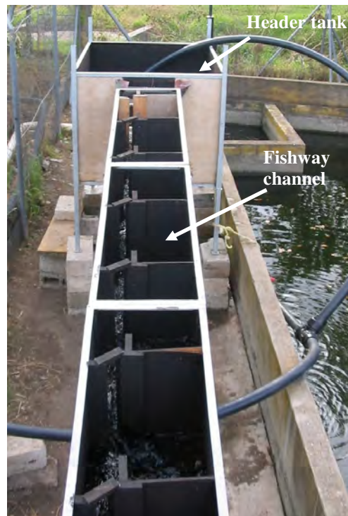
Plate 2.1: Vertical Slot Fishway used during experiments.
