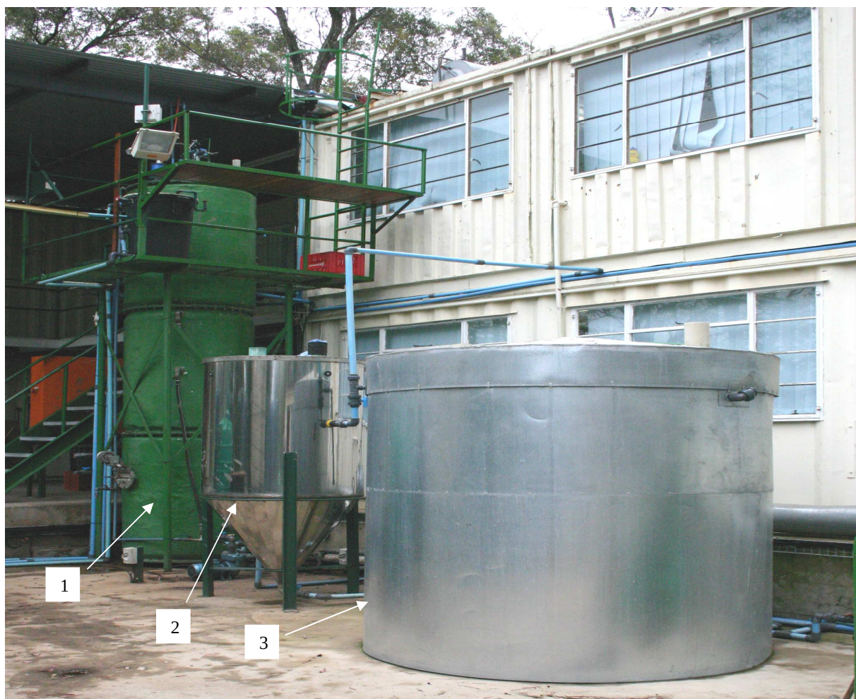
Figure 4.2 Photograph of the Pilot-scale Multi-stage Reactor at Environmental Biotechnology Research Unit (EBRU), Grahamstown South Africa. 1= Column Upflow Recycling Sludge Bed Reactor (RSBRc); 2= Continuous Stirred Tank Reactor (STR); 3= Clarifier.
