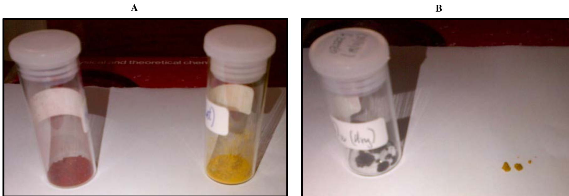
Figure 2.1: Photographs showing the red \rightarrow yellow hydration-induced colour change as [\text{Fe}_n(\mu_{1,1}\text{-pyzNO})_{2n-2}(\text{pyzNO})_{3n+2}](\text{ClO}_4)_{2n} ( n = \{1, 2\} ) (Complex1) transforms to \{\text{Fe}(\text{pyzNO})_5(\text{ClO}_4)_2(\text{H}_2\text{O})_3\} (Complex5) (A); and as [\text{Fe}_{2n}(\mu_{1,5}\text{-pyzNO})_{2n-1}(\text{pyzNO})_{8n+1}](\text{ClO}_4)_{4n} (Complex2) transforms to [\text{Fe}(\text{pyzNO})_4(\text{H}_2\text{O})_2](\text{ClO}_4)_2 \cdot 2\text{H}_2\text{O} (Complex6) (B).
