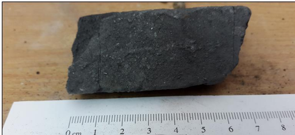
Figure 11: Photograph showing dark graphitic schist with disseminated pyrite; All lengths are in centimetres
