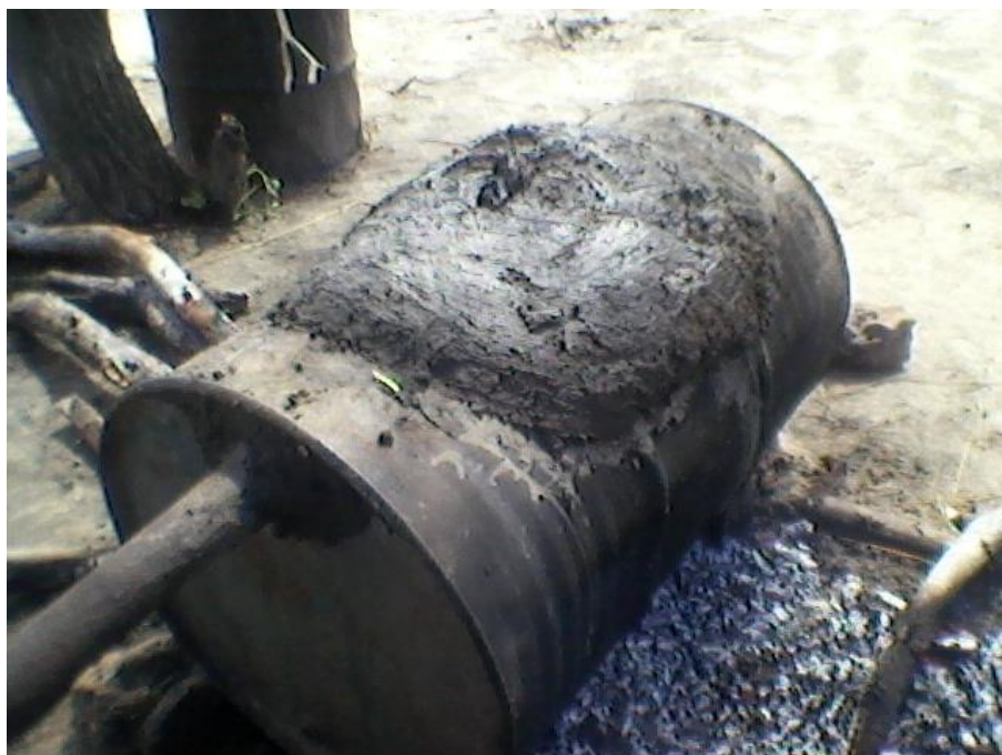
Figure 5.3 (h) Boiling metal drum covered with zinc sheet and mud, distillation process of Kashipembe taking place. ( Ndoroma vana turako sipereki nokuyiramba nosighuru kunakukendja Kashipembe ).
