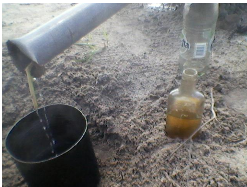
Figure 5.3 (i) Collecting alcohol Kashipembe in a cut can container through the condenser and putting it in a bottle. ( Kuna kughupako marovhu gha Kashipembe musitoromani kupitira mumuyengo makura kugha tura mulikende.
