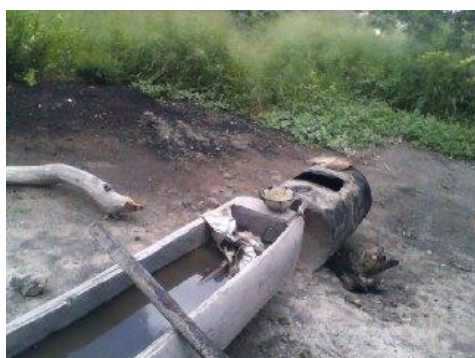
Figure 5.3 (h) Boiling metal drum covered with zinc sheet and mud, distillation process of Kashipembe taking place. ( Ndoroma vana turako sipereki nokuyiramba nosighuru kunakukendja Kashipembe ).
