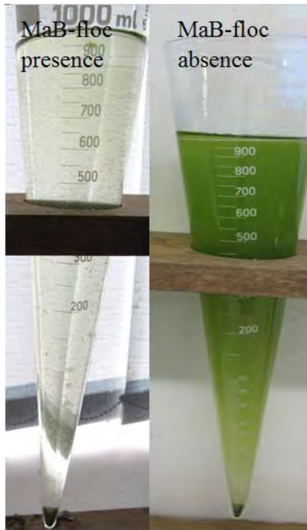
Figure 3:17: Settleability of microalgal bacterial biomass in high rate algae oxidation ponds of an integrated algae pond system treating municipal sewage. 1hr settling time Imhoff cone image during MaB-floc presence and MaB-floc absence.
