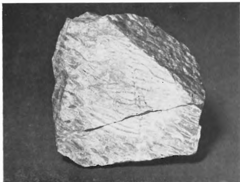
B. Microcline-perthite from the Bold Mine showing albite interlamination. Natural size.
