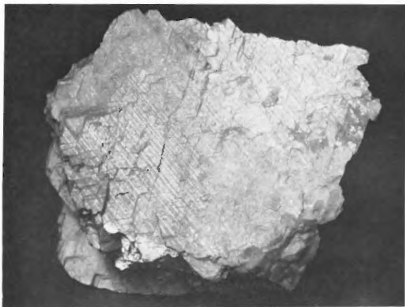
A. Albite from the Early Bird Mine showing polysynthetic twinning. Natural size.
