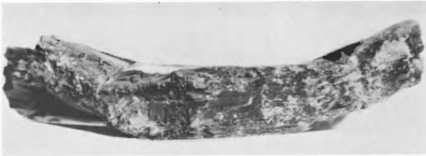
B. Prismatic view of same muscovite crystal A, showing bending as a result of forces set up by replacement of the albite matrix by microcline.
