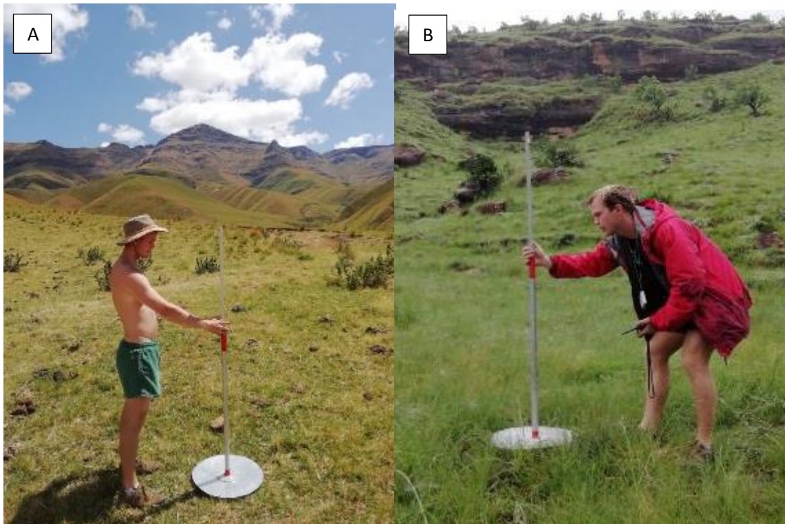
Figure 3.4: Measuring biomass in the Little Pot River catchment with a disk pasture meter. Image A shows low biomass in October 2018 and image B shows higher biomass (in January 2019) than image A (Photo credit: Gareth Snyman (Image A) and Paul Dutton (Image B)).
