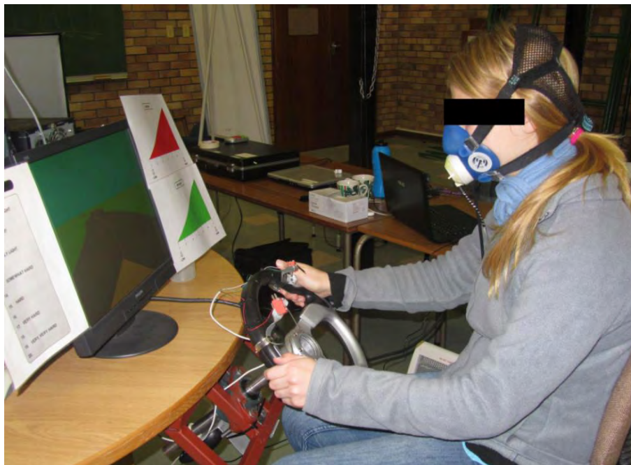
Figure 15: Physical set-up of task alternation experiment displaying participant driving with ergospirometric equipment.
