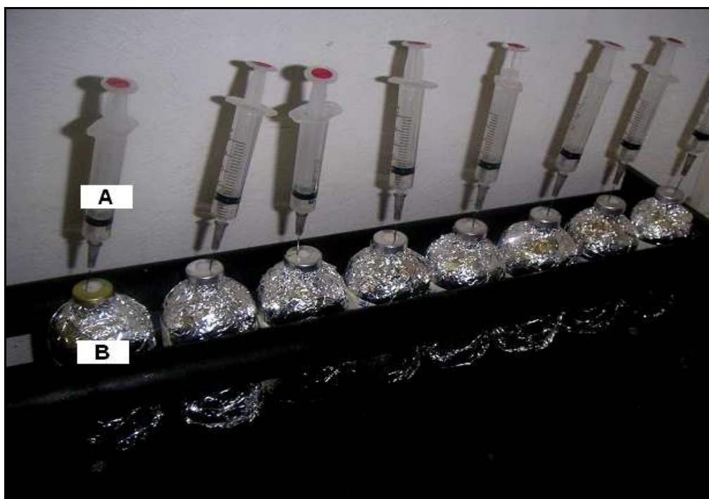
Figure 4.1 Serum bottles used in preliminary studies. (A) Syringe; (B) Serum bottle containing 5 % (w/v) milled grass, C. beijerinckii and 300 \text{ mg l}^{-1} sulphide (test), or 5 % (w/v) milled grass, C. beijerinckii (control 1), or 5 % (w/v) milled grass and 300 \text{ mg l}^{-1} sulphide (control 2), or 5 % (w/v) milled grass (control 3). All were made in 0.1 M phosphate buffer, pH 8 and in duplicate.
