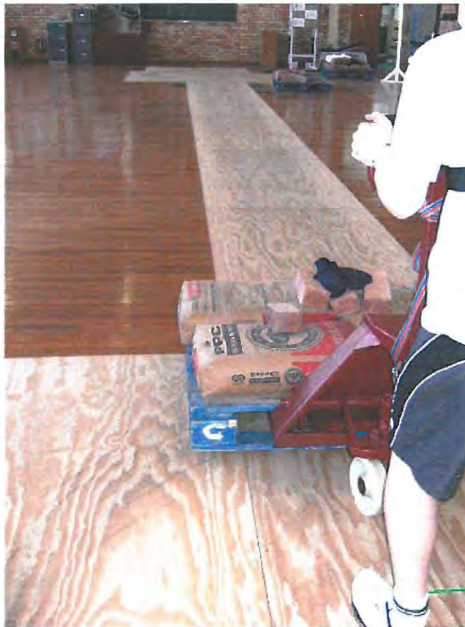
Figure 6: Plywood floored runway used to replicate coefficient of friction evident in flooring used in industry.
