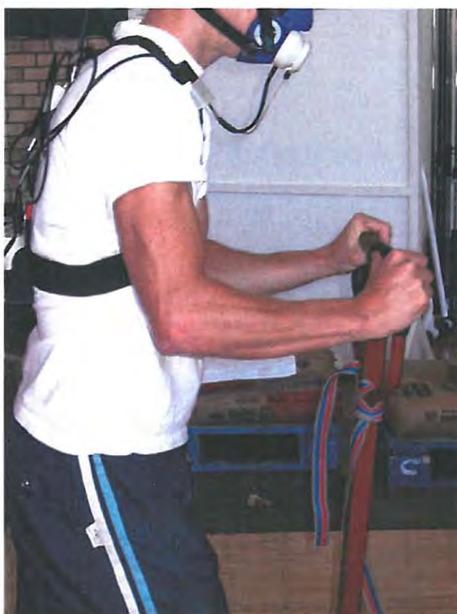
Figure 4: Interaction between desired anthropometry and MHD design allows subjects to exert push forces in positions of optimal strength at approximately elbow height.
