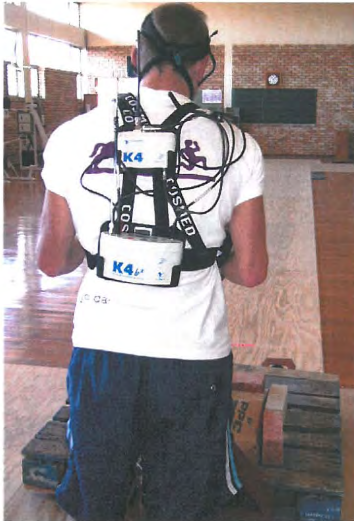
Figure 7: K4b 2 Ergospirometer in use, securely fastened to the subject's back.
