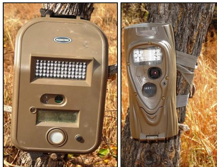
Fig 3.3: Images of the two models of cameras used in the camera trapping survey at Debshan ranch from 20 May to 28 July 2014, Moultrie (left) and Cuddeback (right).
